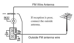
Before attaching a 75 ohm coaxial lead (the kind with a round wire going to an outside antenna), disconnect the supplied FM Wire Antenna.
